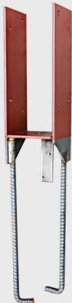
Set the post brackets. The brackets that attach the posts to the concrete piers are wet-set into the concrete and aligned to stringlines indicating the building footprint. Setting up the strings correctly and placing the post bases accurately is crucial for getting a straight, square building.
